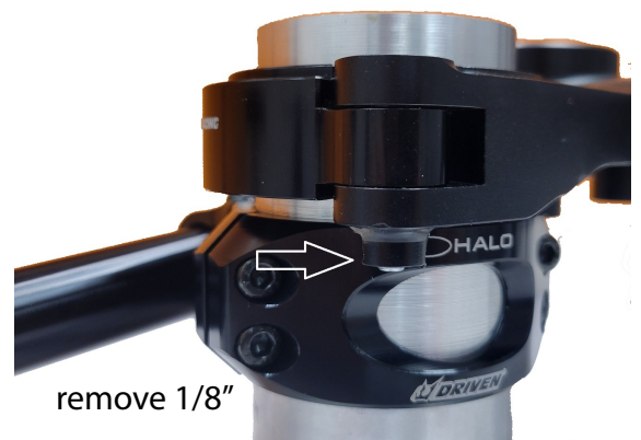
CORRECT (Clamp have 100% fork leg engagement).
