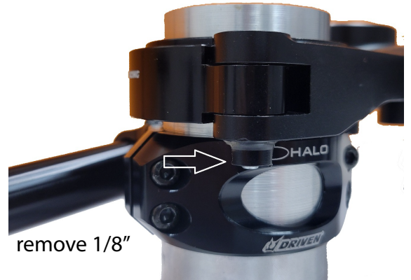
CORRECT (Clamp have 100% fork leg engagement).
